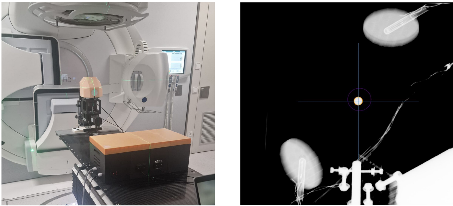
Figure 3 & 4 to the left: Our phantom on the treatment couch (left) & X-ray image of phantom by the ETD SD tool
