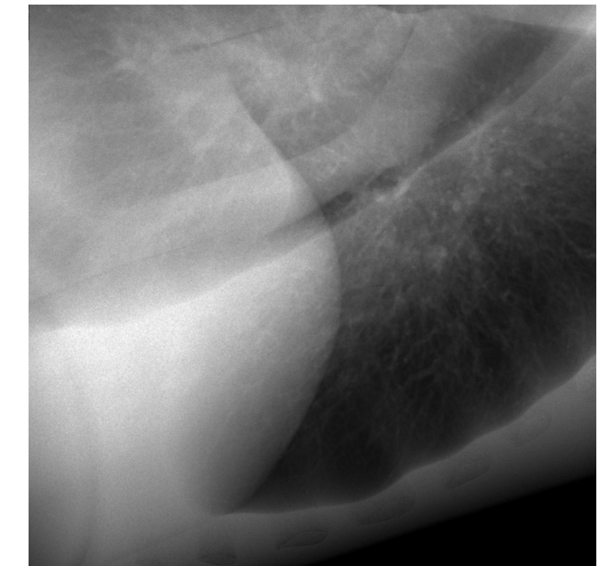
Figure 2 Soft-tissue basis image of the Lungman phantom obtained by DE decomposition using a 60/125 kV acquisition pair with 2 mm Sn filtration at HE
