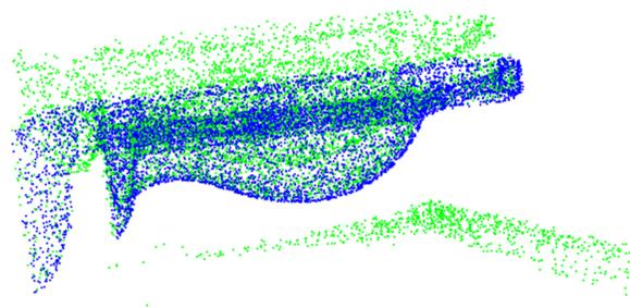
Figure 1: Result of the point cloud registration with the CPD algorithm; green: point cloud created from CT; blue: point cloud created from 4Pi CAD file
